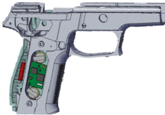
Figure 2. RuBee tag embedded in Sig Sauer P226 Grip
