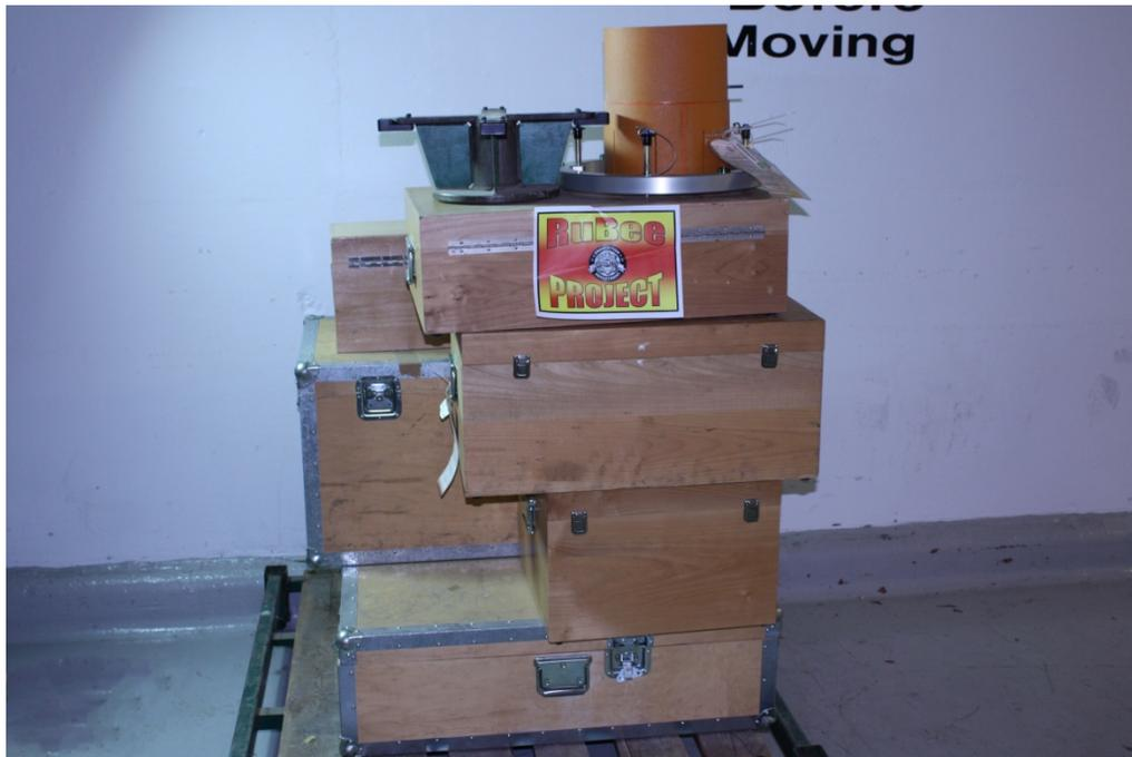
Data was collected regarding the movement and stationary inventory of the selected tool set; including, movement to and from the storage location. Approximately 10 test cycles were conducted to evaluate the performance of the RuBee tags and system. During these cycles, the tagged tools were moved into and out of the interlock loops, and identification accuracy was determined with each inventory.
