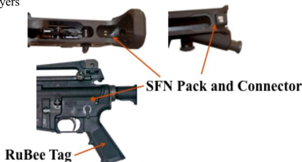
Figure 5 - Tag authentication and part identity is possible with SFN packs, EEPROM 32 bit ID's. The RuBee tag is placed on the lower receiver in the grip, and an SFN tag is placed on the upper receiver and barrel assembly.
